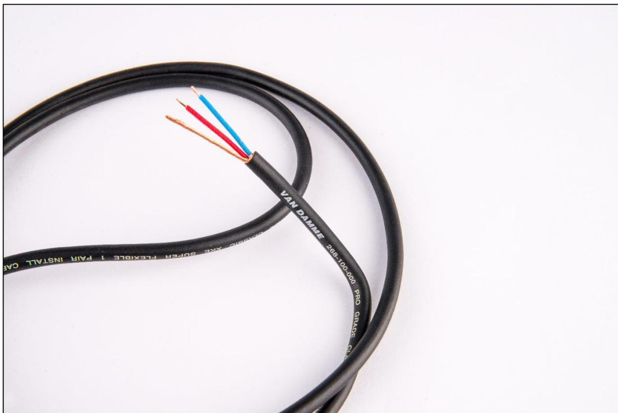
Van Damme Super Flexible 1 pair is a 3.60 mm balanced analogue audio cable with a lapped copper spiral screen. This cable is ideal for use with miniature connectors such as the Switchcraft Tini-Qg range and other small connectors typically found on Lavalier microphones. Its helical spiral shield can withstand multiple flexing operations making it preferable to foil screened 1 pair for certain dynamic applications.
