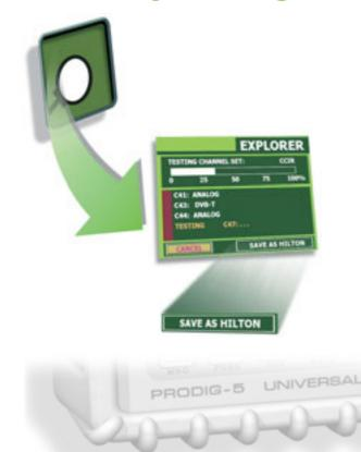
When the 'explorer' key is pressed for a few seconds, a new spectrum exploration session begins. Unlike any other meter currently on the market, the EXPLORER makes a dynamic exploration of the spectrum, detecting all the channels in the swept band. This applies to the terrestrial and satellite television bands.
